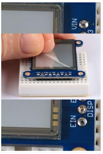
Remove the Protective Film After soldering is complete. Gently peel the film from the display.
