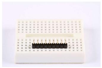
Position the header Trim the header to length if necessary and place it long pins down in your breadboard.
