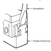
When mounting the Terminal Protective Cover to the case, align the cover on the case and then press the cover down to mount it firmly.
