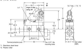
Note: 1. Unless otherwise specified, a tolerance of  $\pm 0.4$  mm applies to all dimensions.
