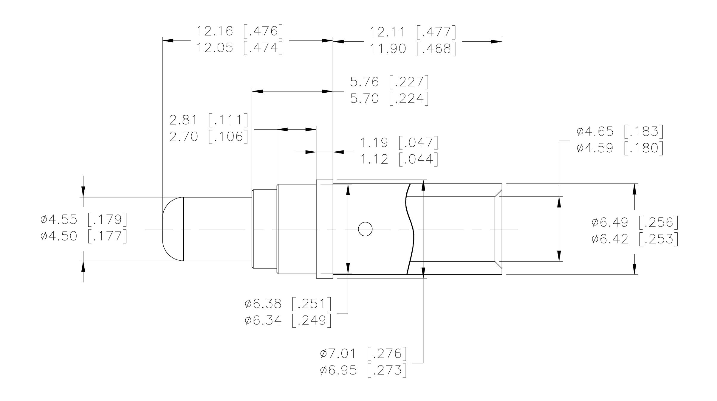
COPPER ALLOY PER ASTM B301
