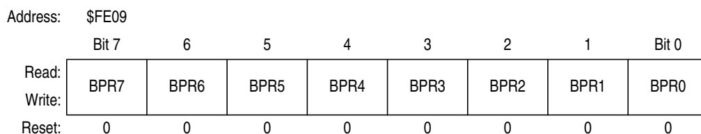
Figure 2-5. FLASH Block Protect Register (FLBPR)
