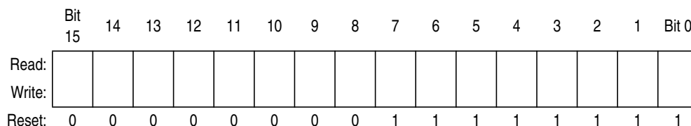
Figure 4-4. Stack Pointer (SP)
