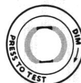
Shutters closed Minimum indirect "halo" light
