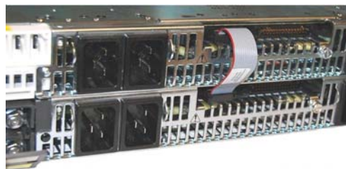
Shelf-to-shelf cable connection (part # CC848848952)
