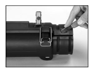
Then place a heavy duty cable tie, hose clamps or metal banding through the slit on each end and tighten to secure and compress seal.
