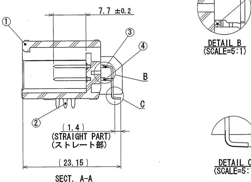
NOTE1. THE TIP OF THE TERMINAL SHALL BE CLOSER (0~0.2) THAN THE BOTTOM TO PCB.
