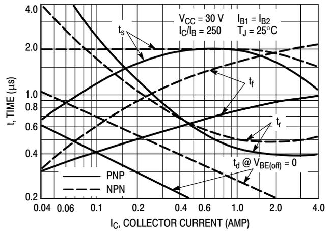
Figure 3. Switching Times
