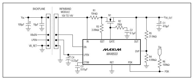
Figure 2. Typical 50W Applications Circuit
