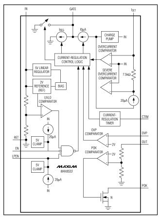
Figure 1. MAX8533 Functional Diagram
