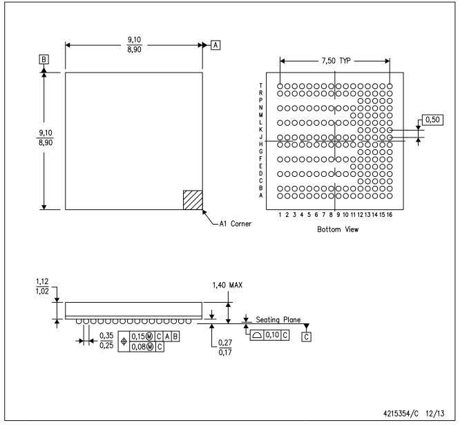
NOTES: A. All linear dimensions are in millimeters. Dimensioning and tolerancing per ASME Y1.5M—1994.
