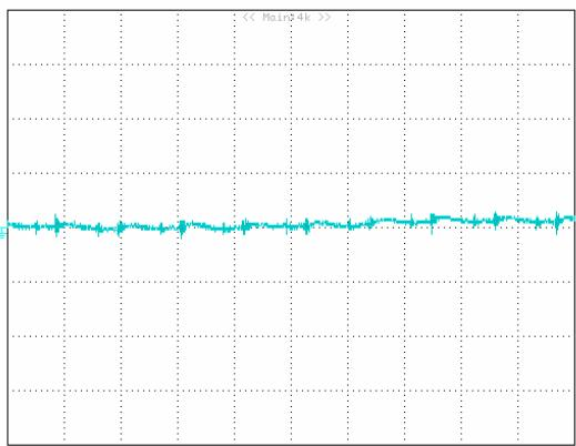
**Figure 13:** Input reflected ripple current,  $i_s$ , through a  $12\mu\text{H}$  source inductor at nominal input voltage and rated load current (20 mA/div, 2μs/div).
