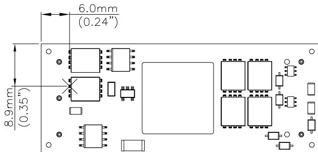
**Figure 18:** Temperature measurement location
