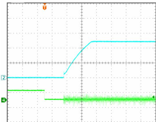
**Figure 6:** Turn-on transient at full rated load current (constant current load) (10 ms/div). Vin=48V. Top Trace: Vout, 5V/div; Bottom Trace: ON/OFF input, 5V/div
