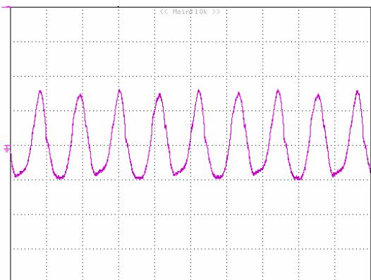
**Figure 12:** Input Terminal Ripple Current,  $i_c$ , at full rated output current and nominal input voltage with  $12\mu H$  source impedance and  $100\mu F$  electrolytic capacitor (200 mA/div, 2us/div).
