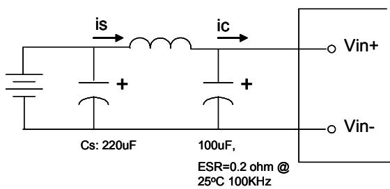
**Figure 11:** Test set-up diagram showing measurement points for Input Terminal Ripple Current and Input Reflected Ripple Current.
