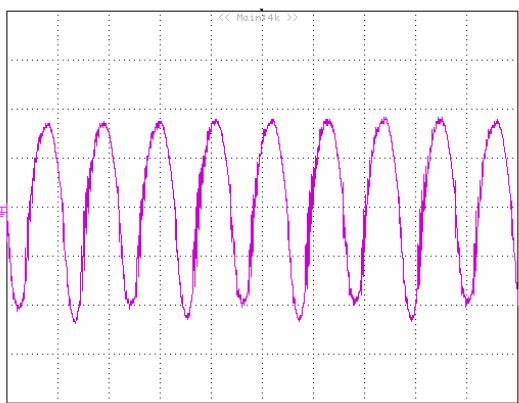
**Figure 15:** Output voltage ripple at nominal input voltage and rated load current ( $I_o=20\text{A}$ ) (20 mV/div, 2μs/div)
