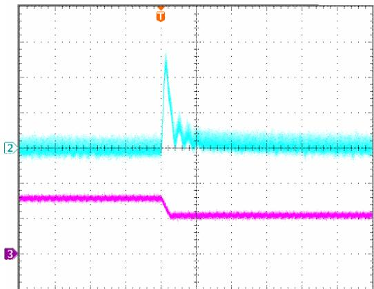
**Figure 9:** Output voltage response to step-change in load current (75%-50% of  $Io$ , max;  $di/dt = 0.1A/\mu s$ ,  $Vin=48V$ ). Load cap:  $10\mu F$ , tantalum capacitor and  $1\mu F$  ceramic capacitor. Top Trace:  $Vout$  (80mV/div, 200us/div); Bottom Trace:  $Io$  (10A/div, 200us/div). Scope measurement should be made using a BNC cable (length shorter than 20 inches). Position the load between 51 mm to 76 mm (2 inches to 3 inches) from the module..
