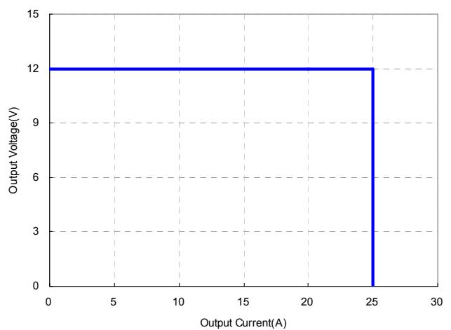
**Figure 4:** Output voltage regulation vs load current showing typical current limit curves and converter shutdown points for minimum, nominal, and maximum input voltage at room temperature
