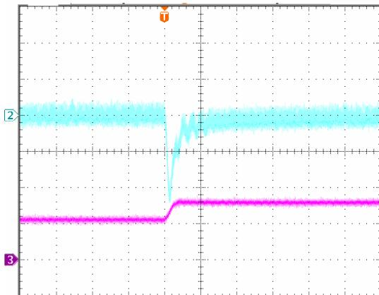
**Figure 10:** Output voltage response to step-change in load current (50%-75% of  $Io$ , max;  $di/dt = 0.1A/\mu s$ ,  $Vin=48V$ ). Load cap:  $10\mu F$ , tantalum capacitor and  $1\mu F$  ceramic capacitor. Top Trace:  $Vout$  (80mV/div, 200us/div); Bottom Trace:  $Io$  (10A/div, 200us/div). Scope measurement should be made using a BNC cable (length shorter than 20 inches). Position the load between 51 mm to 76 mm (2 inches to 3 inches) from the module..
