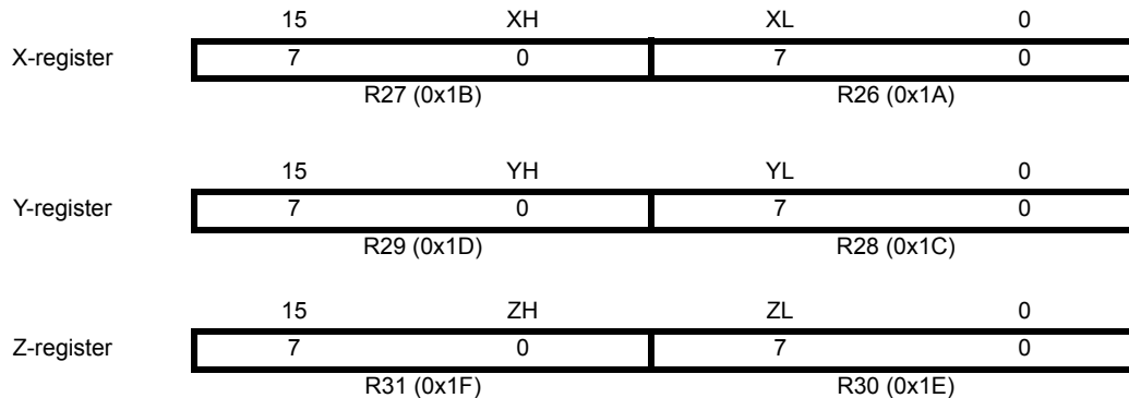
Figure 5-3. The X-, Y-, and Z-registers
