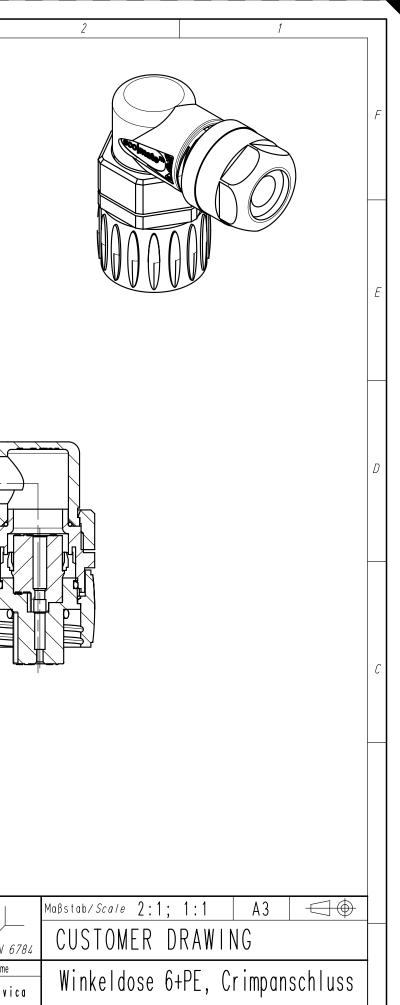
angular female connector, crimp type H M C016 10F006 000 1X - TA
