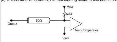
(b) tCHQZ and tCHQX1 are specified with 5pF load capacitance and measured when transition occurs ±100mV from
