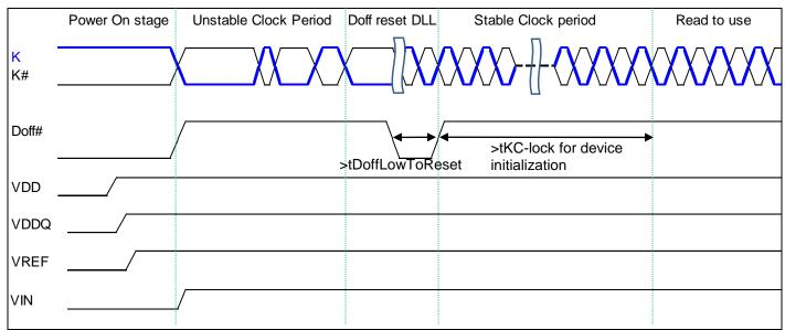
Note) Applying DLL reset sequences (sequence 3a, 3b) are also required when operating frequency is changed without power off.
