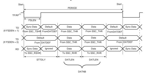
Note: 1. Example of input on falling edge of TF/RF.
