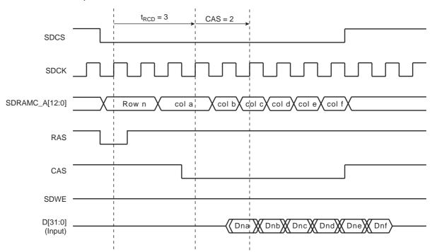
Figure 21-3. Read Burst, 32-bit SDRAM Access
