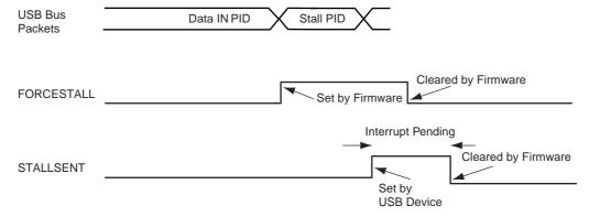
Figure 36-13. Stall Handshake (Data OUT Transfer)
