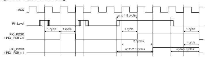
Figure 28-5. Input Glitch Filter Timing
