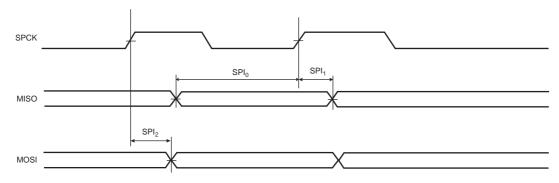
Figure 38-9. SPI Master mode with (CPOL = NCPHA = 0) or (CPOL = NCPHA = 1)
