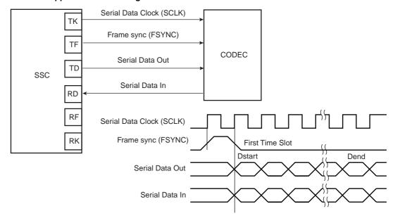
Figure 32-19. Time Slot Application Block Diagram
