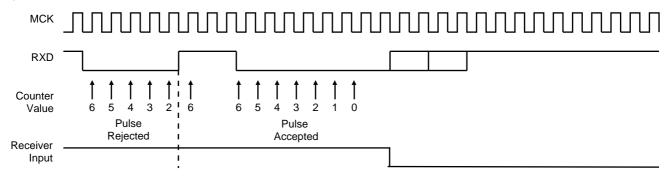
As the IrDA mode uses the same logic as the ISO7816, note that the FI\_DI\_RATIO field in US\_FIDI must be set to a value higher than 0 in order to assure IrDA communications operate correctly.
