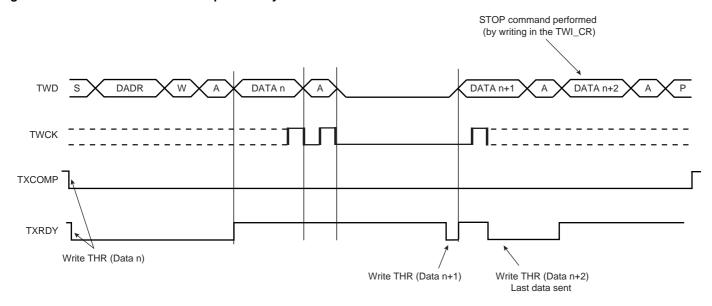
Figure 30-8. Master Write with One Byte Internal Address and Multiple Data Bytes
