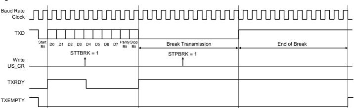
Figure 31-16. Break Transmission
