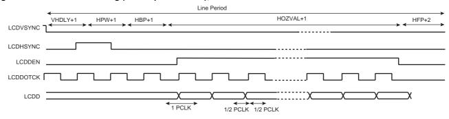
Usually the LCD\_FRM rate is about 70 Hz to 75 Hz. It is given by the following equation:
