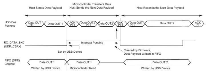
An interrupt is pending while the flag RX\_DATA\_BK0 is set. Memory transfer between the USB device, the FIFO and microcontroller memory can not be done after RX\_DATA\_BK0 has been cleared. Otherwise, the USB device would accept the next Data OUT transfer and overwrite the current Data OUT packet in the FIFO.
