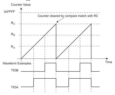
Figure 33-10. WAVSEL = 10 With Trigger
