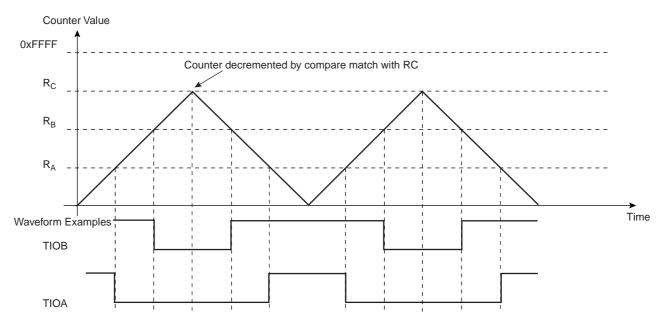
Figure 33-14. WAVSEL = 11 With Trigger
