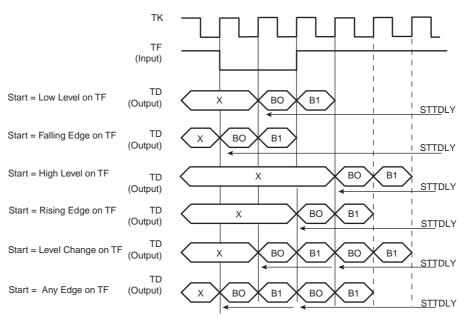
Figure 32-11. Receive Pulse/Edge Start Modes
