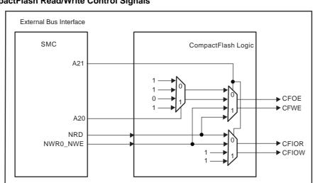
Figure 19-4. CompactFlash Read/Write Control Signals
