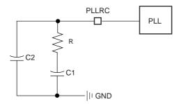
Values of R, C1 and C2 to be connected to the PLLRC pin must be calculated as a function of the PLL input frequency, the PLL output frequency and the phase margin. A trade-off has to be found between output signal overshoot and startup time.
