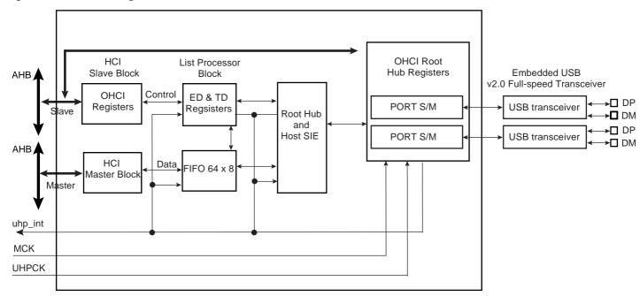
Access to the USB host operational registers is achieved through the AHB bus slave interface. The OpenHCI host controller initializes master DMA transfers through the ASB bus master interface as follows:
