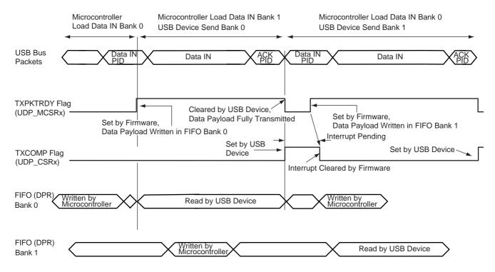
**Warning:** There is software critical path due to the fact that once the second bank is filled, the driver has to wait for TX\_COMP to set TX\_PKTRDY. If the delay between receiving TX\_COMP is set and TX\_PKTRDY is set too long, some Data IN packets may be NACKed, reducing the bandwidth.
