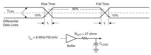
Table 38-24. USB Data Signal Rise and Fall Time Characteristics (Low Speed)
