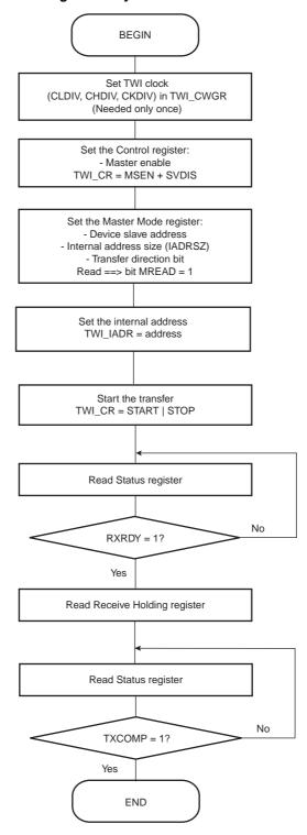
Figure 30-20. TWI Read Operation with Multiple Data Bytes with or without Internal Address
