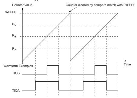
Figure 33-8. WAVSEL= 00 with trigger
