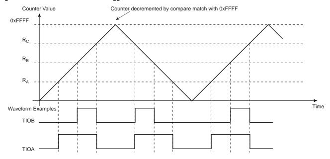
Figure 33-12. WAVSEL = 01 With Trigger
