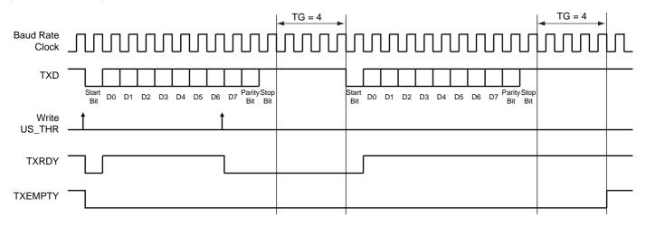
Table 31-7 indicates the maximum length of a timeguard period that the transmitter can handle in relation to the function of the Baud Rate.
