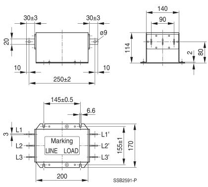
General tolerances according to ISO 2768-cL Dimensions in mm
