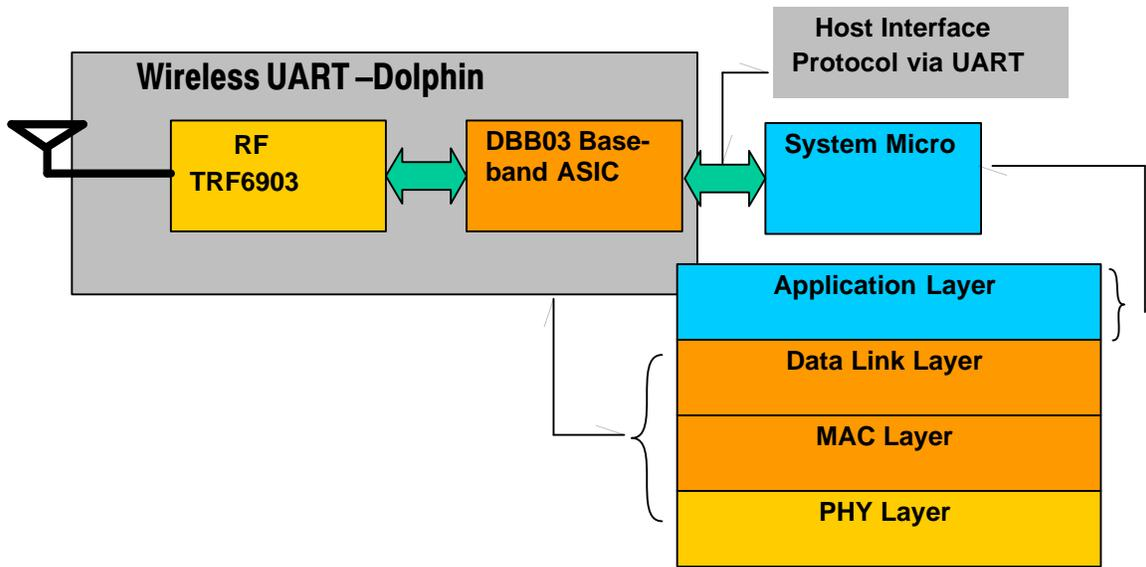
**Figure 1. DBB03 - Baseband ASIC for the Dolphin Chipset**
