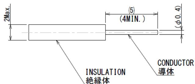
Note 1: Applicable cable (conductor): single wire 26AWG (0.4 Dia.)
