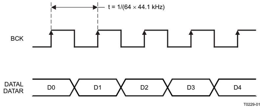
Figure 45. Normal Data Output Form From DSD Decoder
