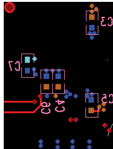
Figure 60. Bottom Layer Decoupling
