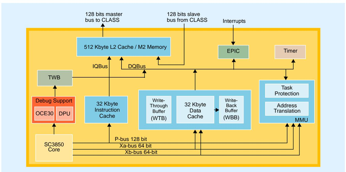
Figure 2. StarCore SC3850 DSP Subsystem Block Diagram
