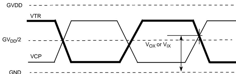
Figure 15. DDR2 and DDR3 SDRAM Differential Timing Specifications
