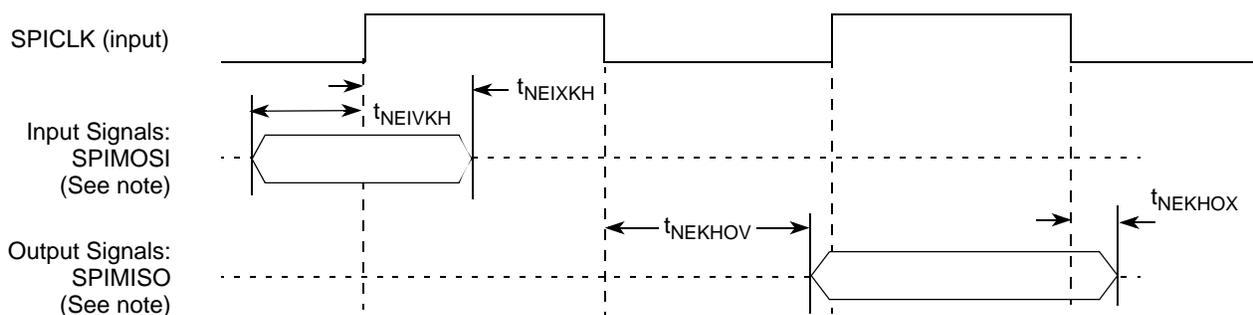
**Note:** measured with  $\text{SPMODE[CI]} = 0$ ,  $\text{SPMODE[CP]} = 0$
