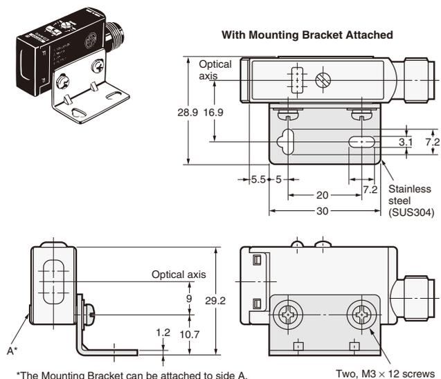
\*The Mounting Bracket can be attached to side A.
