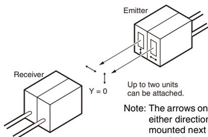
Note: The arrows on the Filters can be attached in either direction when two Sensors are mounted next to each other. The Filter attached to an Emitter and to the corresponding Receiver must be the same in direction of polarization or the Sensor will not function.
