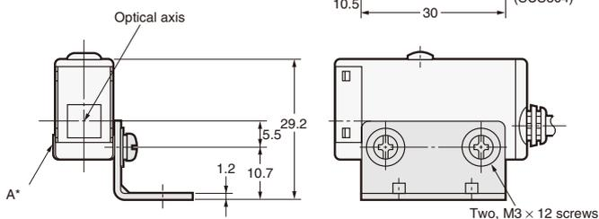
\*The Mounting Bracket can be attached to side A.
