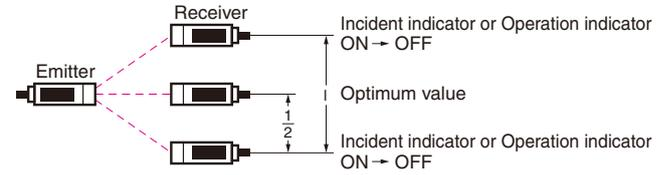
**Optical axis:** The axis from the center of the lens to the center of the beam for the Emitter and the axis from the center of the lens to the center of the reception area for the Receiver.
