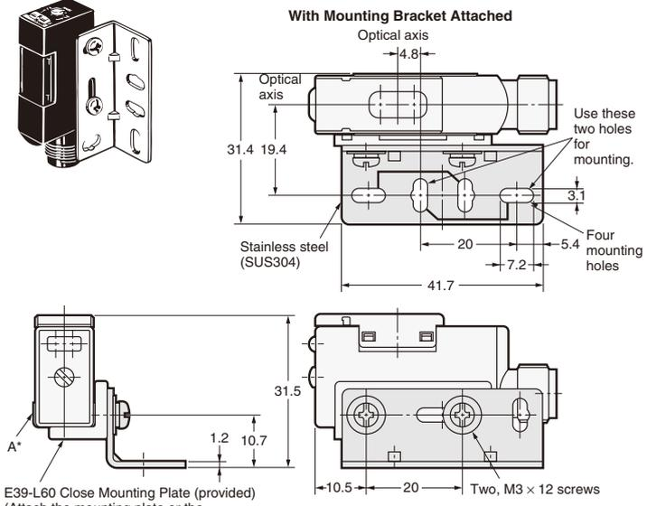
E39-L60 Close Mounting Plate (provided) (Attach the mounting plate or the plug cannot be connected.)
