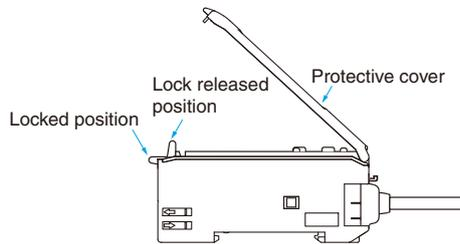
Note: 1. To maintain the fiber characteristics, make sure that the lock is released before removing the fibers.
