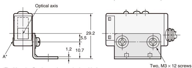
\*The Mounting Bracket can be attached to side A.
