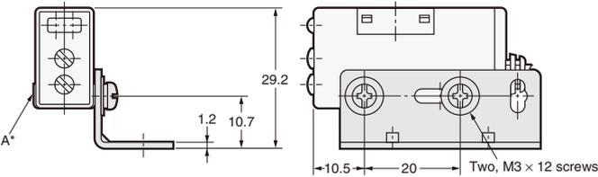
\*The Mounting Bracket can be attached to side A.
