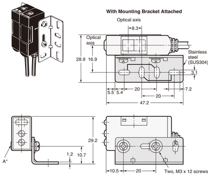
\*The Mounting Bracket can be attached to side A.
