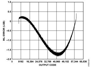
Figure 21. INL with  $f_{IN} = 2.4 \text{ MHz}$
