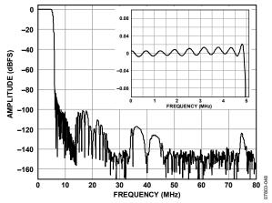
Figure 48. 5 MHz Signal Bandwidth, 160 MSPS
