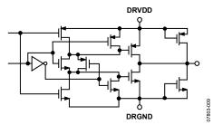
Figure 27. Equivalent Digital Output Circuit
