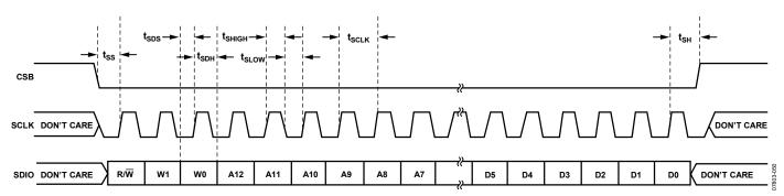
Figure 50. Serial Port Interface Timing Diagram
