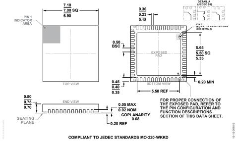
Figure 51. 48-Lead Frame Chip Scale Package [LFCSP] 7 mm × 7 mm Body and 0.75 mm Package Height (CP-48-9) Dimensions shown in millimeters
