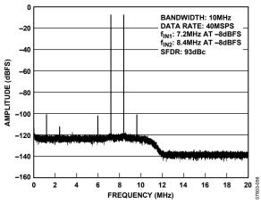
Figure 13. Two-Tone FFT with  $f_{\text{IN1}} = 7.2 \text{ MHz}$  and  $f_{\text{IN2}} = 8.4 \text{ MHz}$
