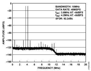
Figure 12. Two-Tone FFT with  $f_{\text{IN1}} = 3.6 \text{ MHz}$  and  $f_{\text{IN2}} = 4.2 \text{ MHz}$
