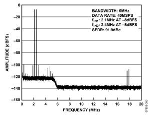
Figure 7. Two-Tone FFT with  $f_{\text{IN1}} = 2.1$  MHz,  $f_{\text{IN2}} = 2.4$  MHz and BW = 5 MHz
