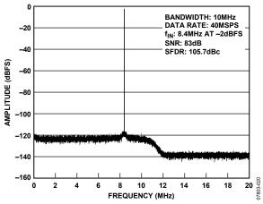
Figure 10. Single-Tone FFT with  $f_{IN} = 8.4 \text{ MHz}$
