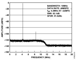
Figure 9. Single-Tone FFT with  $f_{IN} = 4.2 \text{ MHz}$
