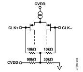
Figure 23. Equivalent Clock Input Circuit
