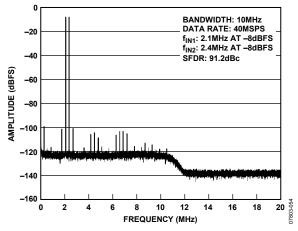
Figure 11. Two-Tone FFT with  $f_{\text{IN1}} = 2.1$  MHz and  $f_{\text{IN2}} = 2.4$  MHz
