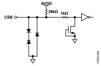
Figure 26. Equivalent CSB Input Circuit
