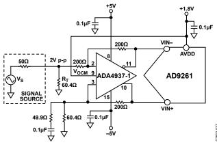
Figure 37. Differential Input Configuration Using the ADA4937-1
