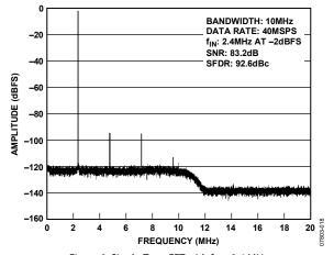
Figure 8. Single-Tone FFT with  $f_{IN} = 2.4 \text{ MHz}$
