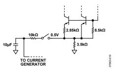
Figure 28. Equivalent VREF Circuit
