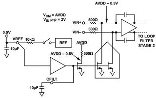
Figure 39. Voltage Reference Loop
