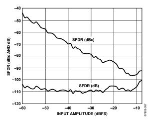
Figure 15. Two-Tone SFDR/IMD3 vs. Input Amplitude with  $f_{\text{IN1}} = 2.1 \text{ MHz}$  and  $f_{\text{IN2}} = 2.4 \text{ MHz}$
