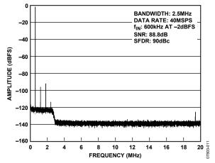
Figure 4. Single-Tone FFT with  $f_{IN} = 600 \text{ kHz}$  and BW = 2.5 MHz
