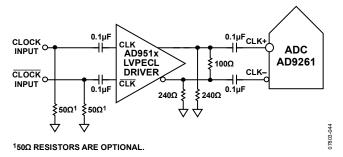
Figure 44. Differential LVPECL Sample Clock
