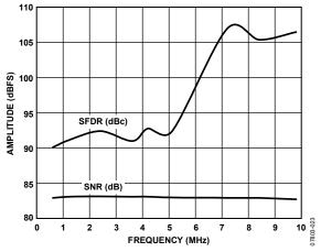
Figure 17. SNR/SFDR vs. Input Frequency
