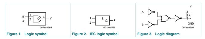
Low-power 2-input AND gate with open-drain
