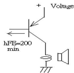
The base current  $I_b$  should be high enough so that it saturates the collector current of the transistor with the CB load.
