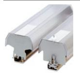
Cover profile, for covering terminal strips, snaps onto cover profile carrier AP 3-TU, AP 3-TNS 35, can be marked with insert strip AP-ES. Cover profile carriers should be placed at the ends and at intervals of approx. 40 cm. Length: 1 m
