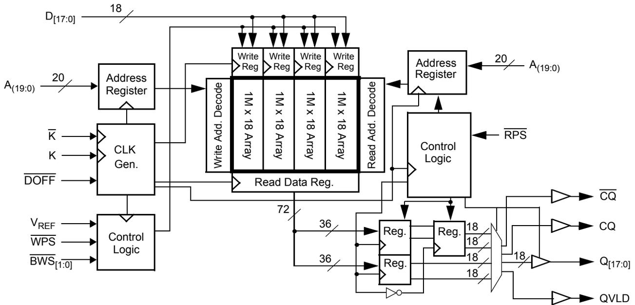
**Logic Block Diagram – CY7C1545KV18**
