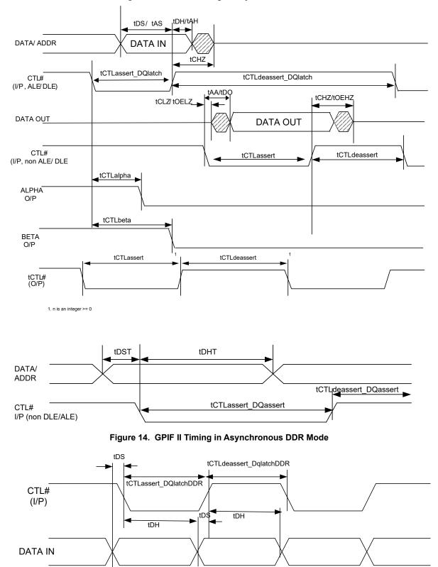
Figure 13. GPIF II Timing in Asynchronous Mode
