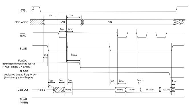
Figure 26. Asynchronous Slave FIFO Read Mode
