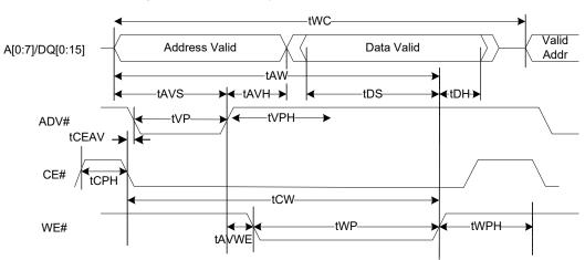
Figure 19. ADMux Asynchronous Random Write
