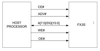
FX3S's ADMux interface supports a 16-bit time-multiplexed address/data SRAM bus.
