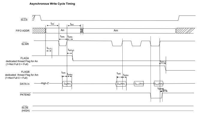
tWRPE: SLWR# de-assert to PKTEND deassert = 2ns min (This means that PKTEND should not be be deasserted before SLWR#) Note: PKTEND must be asserted at the same time as SLWR#.
