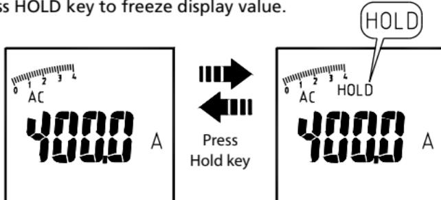
**SMART HOLD:** The meter will beep continuously and the display will flash if the measured signal is larger than the display reading. (for V.A.W function)
