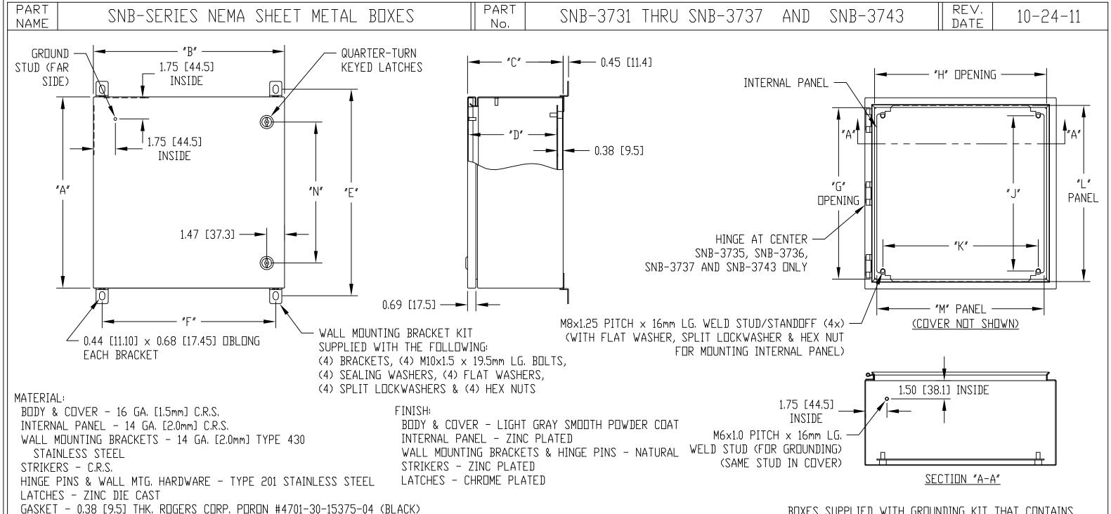
BOXES SUPPLIED WITH GROUNDING KIT THAT CONTAINS THE FOLLOWING: (1) GROUND WIRE, (4) FLAT WASHERS, (2) SPLIT LOCKWASHERS AND (2) HEX NUTS
