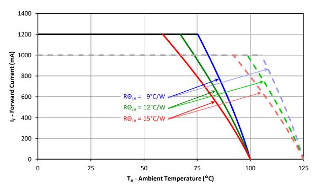
Figure 10: Maximum forward current vs. ambient temperature
