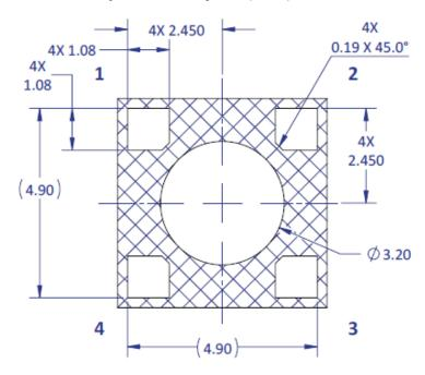
Figure 2c: Recommended solder mask opening for anode, cathode, and thermal pad for non-pedestal and pedestal design
