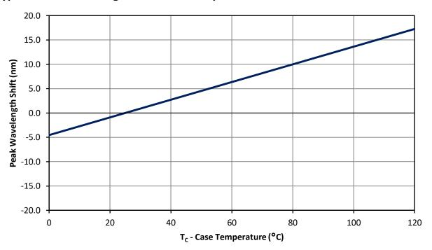
Figure 9: Typical peak wavelength shift vs. case temperature.
