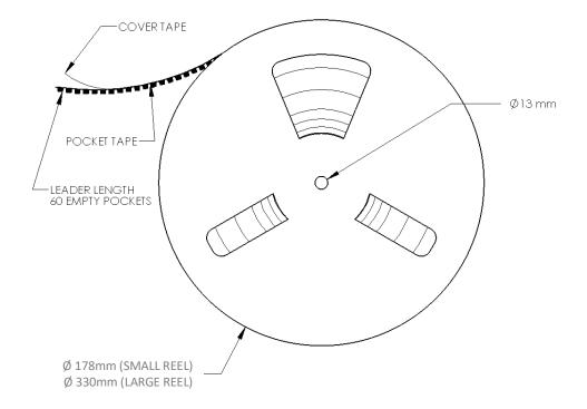
Figure 12: Emitter reel specifications (mm).
