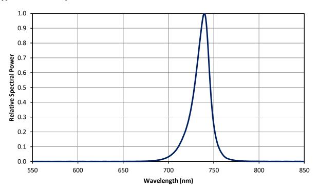
Figure 5: Relative spectral power vs. wavelength @  $I_F$  = 350mA and  $T_C$  = 25°C.
