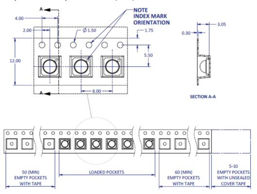
Figure 11: Emitter carrier tape specifications (mm).
