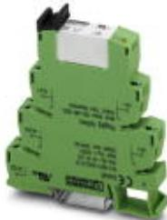
PLC-INTERFACE, consisting of PLC-BPT.../21-21 basic terminal block with push-in connection and plug-in miniature relay with multi-layer gold contact, for mounting on DIN rail NS 35/7,5, 2 PDTs, input voltage 120 V AC/DC
