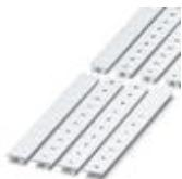
Zack marker strip, Strip, white, labeled, can be labeled with: Plotter, Printed horizontally: Consecutive numbers 1 - 10, 11 - 20, etc. up to 991 - 1000, Mounting type: Snap into tall marker groove, for terminal block width: 10.2 mm, Lettering field: 10.15 x 10.5 mm
