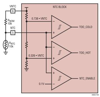
Figure 8. Typical NTC Thermistor Circuit
