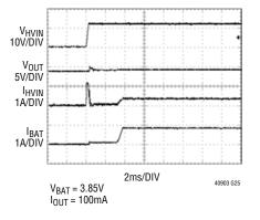
LTC4090 High Voltage Input Disconnect Waveforms
