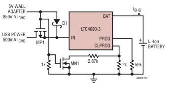
Figure 4. USB or 5V Wall Adapter Power
