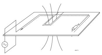
Figure 11. Ground Currents Follow Their Incident Path at High Speed. Slices in the Ground Plane Cause High Voltage and Increased Emissions.
