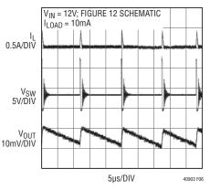
Figure 6. High Voltage Regulator Burst Mode Operation
