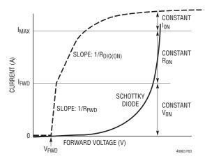
Figure 3. LTC4090-3 vs Schottky Diode Forward Voltage Drop
