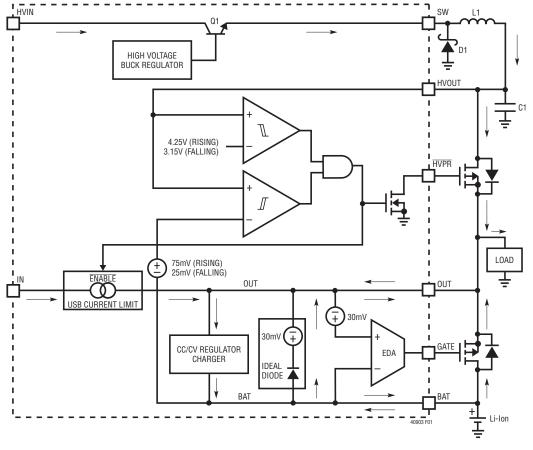
Figure 1. Simplified PowerPath Block Diagram
