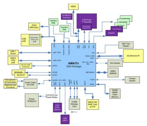
Figure 3. AM437x EVM System Block Diagram
