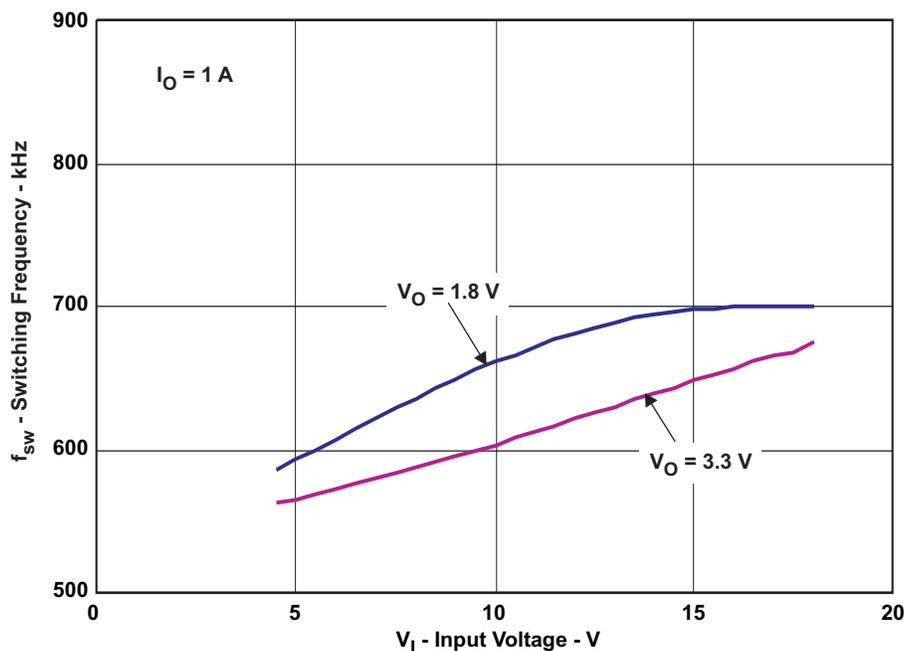
**Figure 8. TPS54225EVM-538 Switching Frequency**
