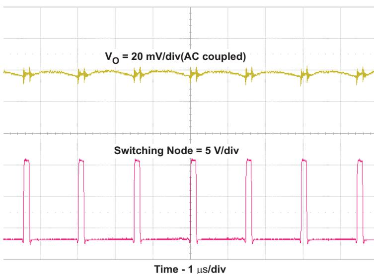
Figure 5. TPS54225EVM-538 Output Voltage Ripple
