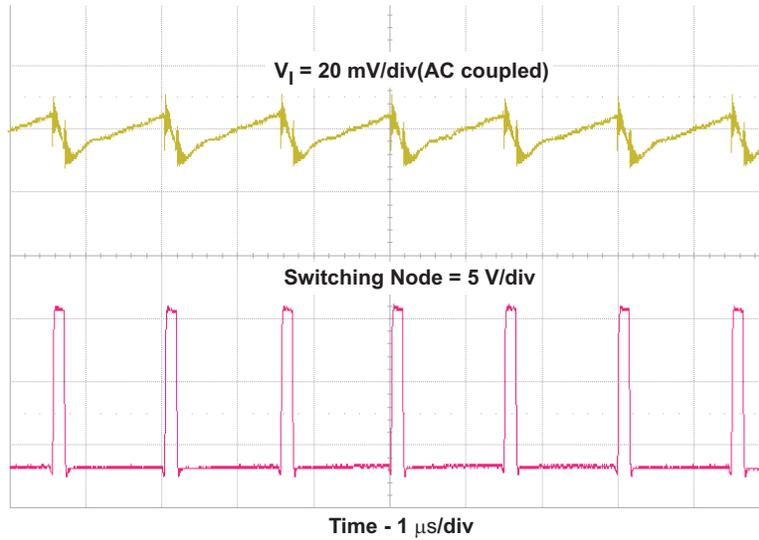
Figure 6. TPS54225EVM-538 Input Voltage Ripple
