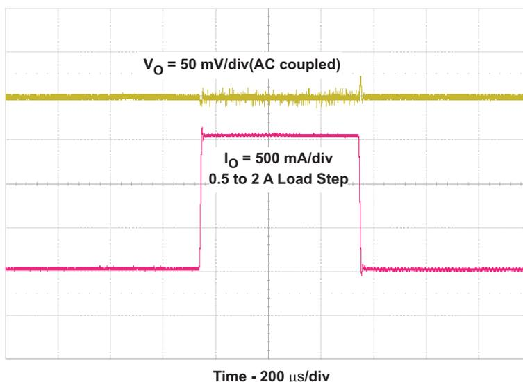
Figure 4. TPS54225EVM-538 Load Transient Response
