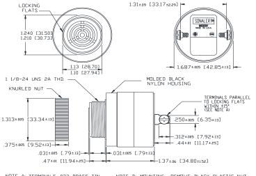
NOTE A: TERMINALS-.032 BRASS TIN PLATED, TAPPED FOR #6-32 SCREW. TWO #6-32 NICKEL PLATED BRASS SCREWS INCLUDED. WILL ACCEPT 1/4" QUICK CONNECT. NOTE B: MOUNTING- REMOVE BLACK PLASTIC NUT AND INSERT THREADED FRINT THROUGH 1.25' HOLE PUNCHED IN PANEL, IF DRIENTATION IS NEEDED, NOTE LOCKING FLATS ON DRAWING. SCREW NUT BACK ON. DO NOT OVERTIGHTEN.
