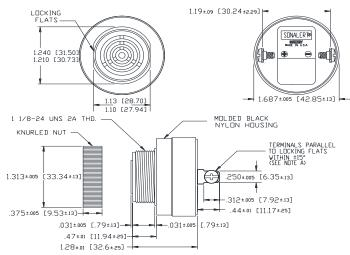
NOTE A: TERMINALS-032 BRASS TIN PLATED, TAPPED FOR #6-32 SCREW. TWO #6-32 NICKEL PLATED BRASS SCREWS INCLUBED. WILL ACCEPT 1/4' QUICK CONNECT. NOTE B: MOUNTING- REMOVE BLACK PLASTIC NUT AND INSERT THREADED FRINT THROUGH 1.25' HOLE PUNCHED IN PANEL, IF DRIENTATION IS NEEDED, NOTE LOCKING FLATS ON DRAVING. SCREW NUT BACK ON. DO NOT OVERTIGHTEN.
