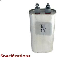
Type SCRN capacitors are for SCR (silicon controlled rectifier) commutating applications that require high peak and rms current capability. These capacitors are ideal for other high frequency and pulsed applications. The SCRN is supplied in oval or rectangular metal cases with  $1/4 \times 20$  threaded stud and insulated terminals to withstand high current and high peak voltages.
