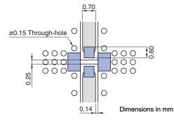
Line width be designed to match  $50\Omega$  characteristic impedance depending on PCB material and thickness.
