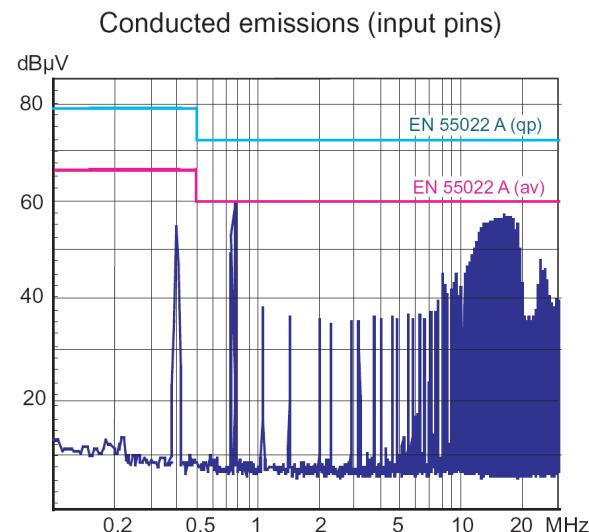
To meet level B, it is necessary to fit a 5  $\mu$ F ceramic capacitor across the input terminals.
