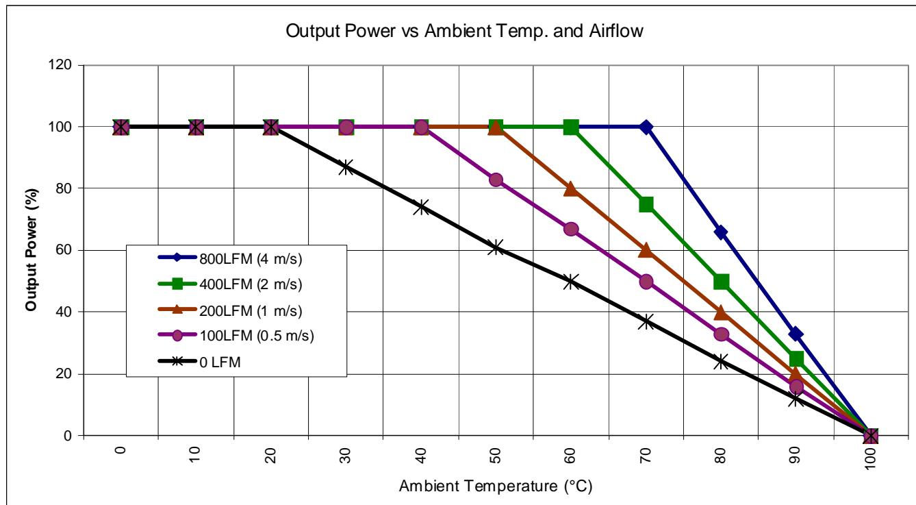
**Note:** For continuous operation above 60 V input, the available output power is further derated linearly up to 50% at 75 V input. This additional derating is due to a predictable drop in efficiency at high input voltage.
