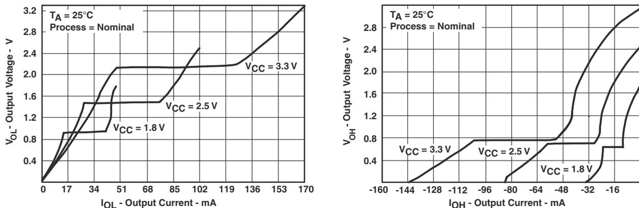
Figure 1. Typical Output Voltage vs Output Current
