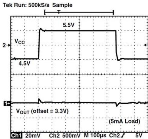
Figure 22. Line Transient (1  $V_{PP}$ ) Response
