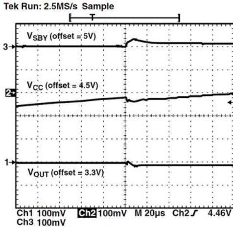
Figure 17.  $V_{CC}$  Power Up
