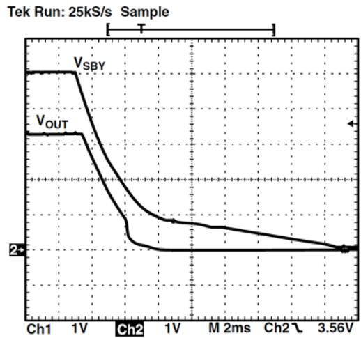
Figure 14.  $V_{SBY}$  Full Power Down (Load = 400 mA)
