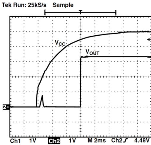
Figure 11.  $V_{CC}$  Cold Start (Load = 400 mA)
