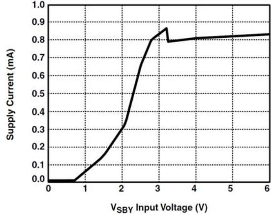
Figure 2. V<sub>SBY</sub> Supply Current vs. Voltage
