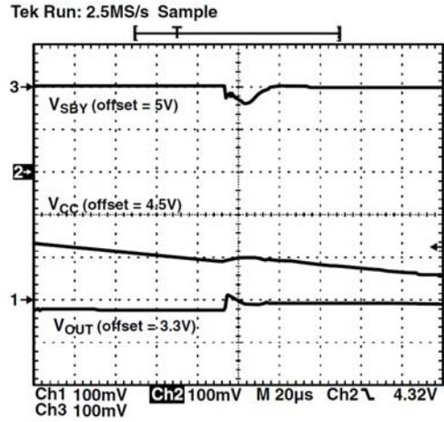
Figure 18.  $V_{CC}$  Power Down
