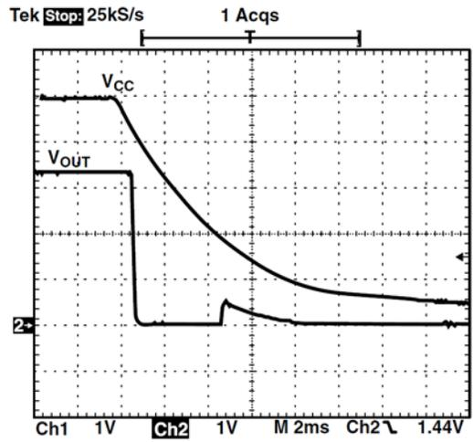
Figure 12.  $V_{CC}$  Full Power Down (Load = 400 mA)
