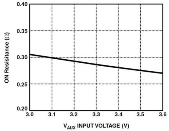
Figure 10. Switch Resistance vs. V<sub>AUX</sub> Supply
