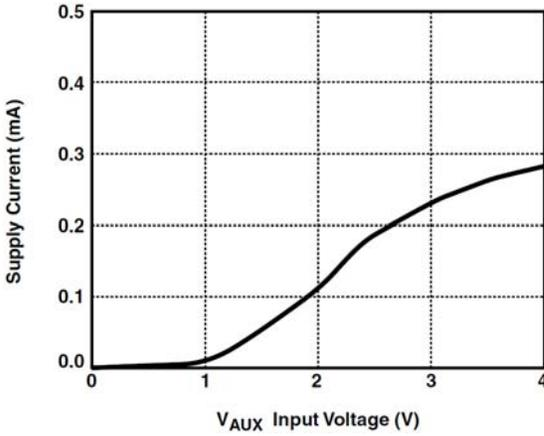
Figure 3. V<sub>AUX</sub> Supply Current vs. Voltage
