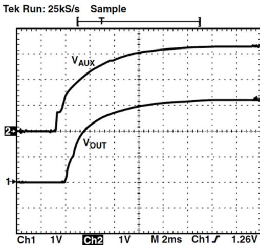
Figure 15.  $V_{AUX}$  Cold Start (Load = 400 mA)
