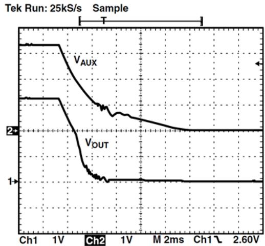
Figure 16.  $V_{AUX}$  Full Power Down (Load = 400 mA)
