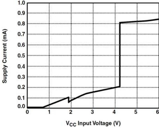
Figure 1. V<sub>CC</sub> Supply Current vs. Voltage
