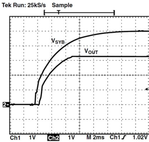
Figure 13.  $V_{SBY}$  Cold Start (Load = 400 mA)
