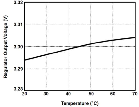
Figure 23.  $V_{OUT}$  Variation with  $T_{AMB}$ (400 mA Load)<sub>T</sub>
