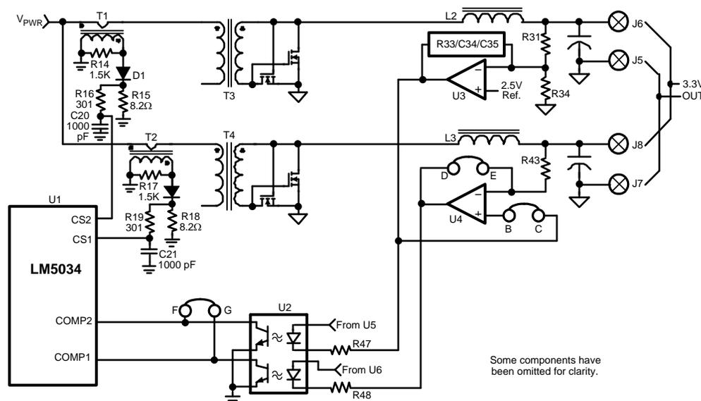
Figure 5. Feedback Configuration for Single High Current Output
