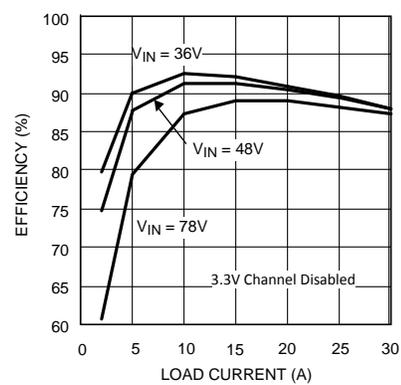
Figure 11. 2.5V Channel Efficiency (Separate Output Configuration)
