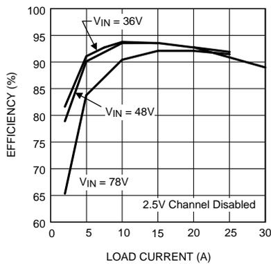
Figure 10. 3.3V Channel Efficiency (Separate Output Configuration)
