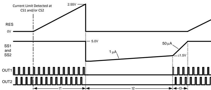
Figure 6. Current Limit Restart Operation
