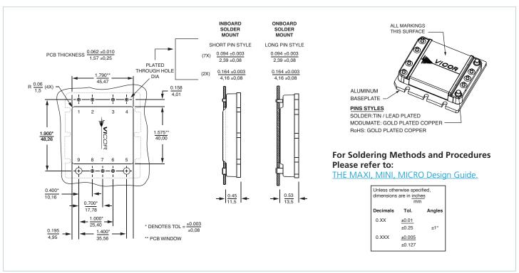
**Figure 13** — PCB mounting specifications
