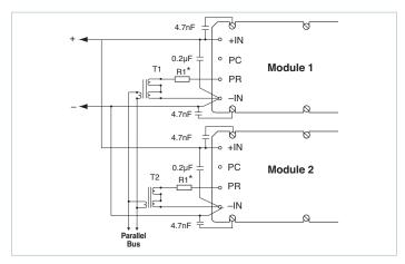
**Figure 10** — Transformer-coupled interface
