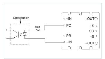
Figure 6 — Isolated on-state indicator
