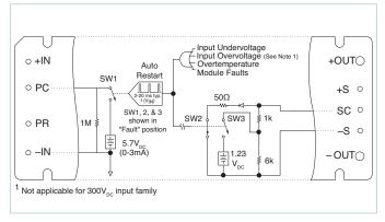
Figure 3 — PC/SC module alarm logic
