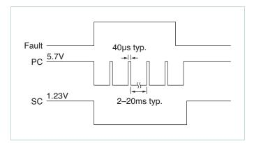
Figure 5 — PC/SC module alarm timing
