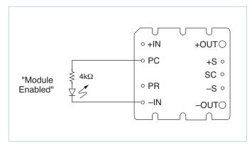
Figure 4 — LED on-state indicator
