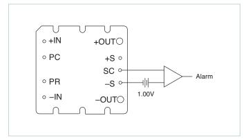
Figure 7 — Secondary side on-state indicator
