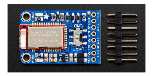
HW flow control (CTS+RTS) should always be used with the nRF51822. The UART peripheral block is designed in a way that more or less requires HW flow control for reliable UART communication, with a very small internal buffer and tight timing limitations due to the SoftDevice architecture (Nordic's proprietary Bluetooth Low Energy stack).
