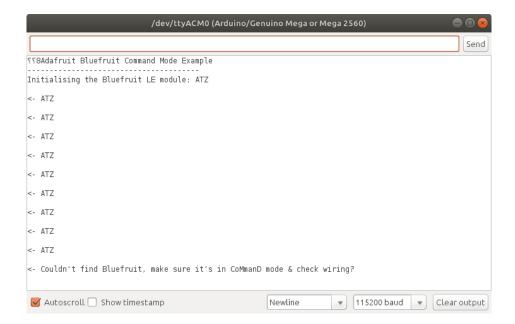
Then double check your wiring and make sure the slide switch is in the CMD position. If that all seems OK, you can also try power cycling the Bluefruit LE UART Friend. Simply remove the 5V wire for a sec and then reconnect it. Then try running the sketch again. Hopefully it'll start responding then.
