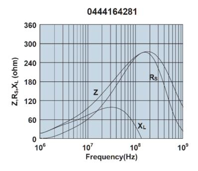
Impedance, reactance, and resistance vs. frequency.
