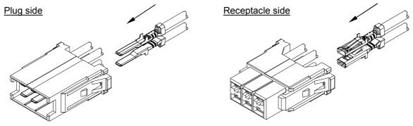
① Please hold the wire at a 10mm distance from the crimped section.
