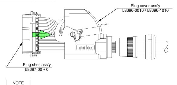
When the cover is installed in the plug shell ass'y the tightening torque of the M2.5 screw is assumed to be 4∼5kgf.
