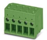
PCB terminal block, nominal current: 32 A, nom. voltage: 630 V, pitch: 7.62 mm, number of positions: 1, connection method: Front screw connection, mounting: Wave soldering, conductor/PCB connection direction: 0 °, color: black. The article can be aligned to create different nos. of positions!
