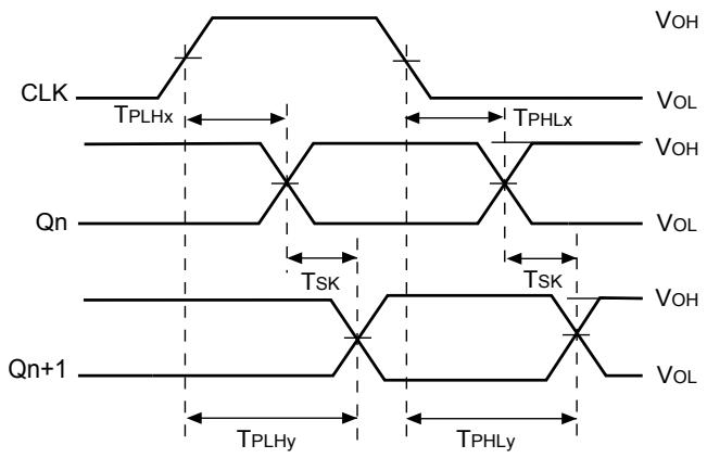
$$T_{SK} = T_{PLHx} - T_{PLHy} \text{ or } T_{SK} = T_{PHLy} - T_{PHLx}$$
