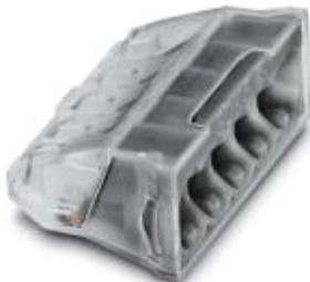
5-pos. socket terminal block with spring-cage connection, for toolless wiring with push-in connection method, for one and multi-strand conductors with a cross section of 0.5 to 2.5 mm<sup>2</sup>, insulation housing transparent.
